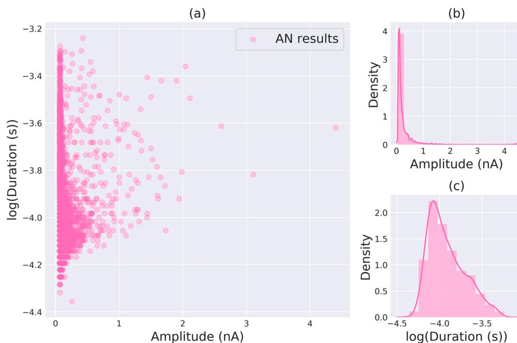
**Figure 3.** Characteristics of the 2111 confident events detected by AutoNanopore on all 23 abf files: (a) scatter plot of the amplitude versus duration of the events; (b) histogram of the amplitude; (c) histogram of the duration.
