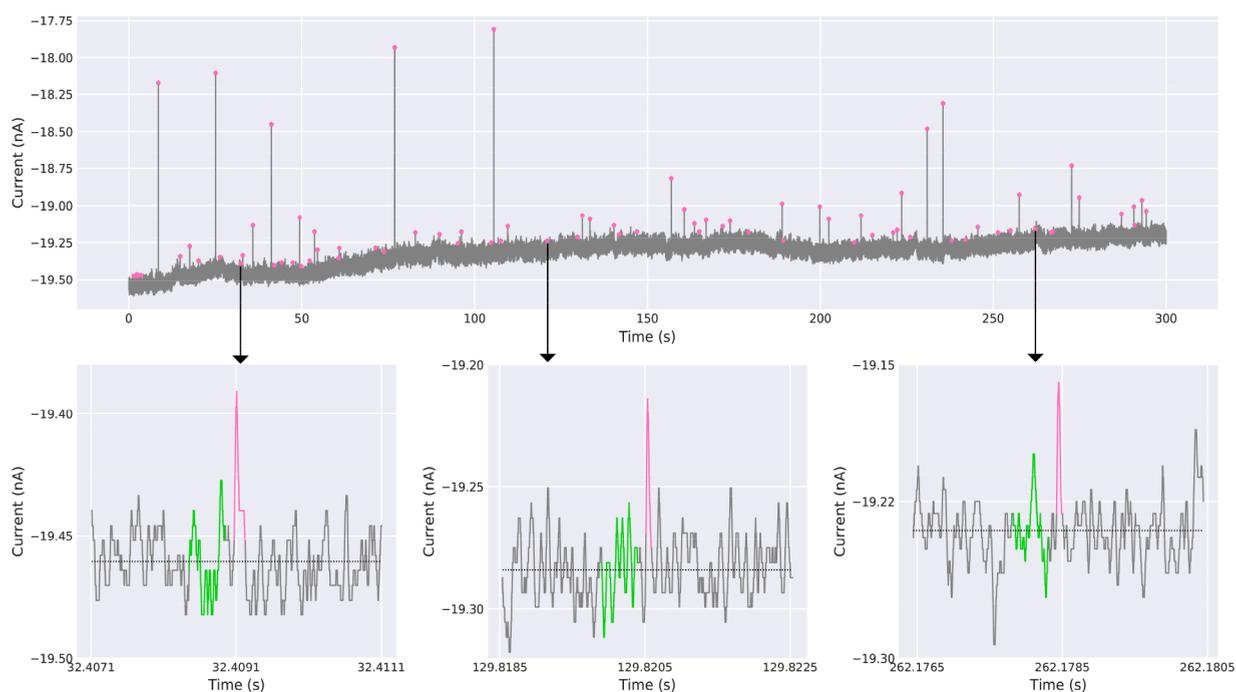
**Figure 2.** Illustration of the events that AutoNanopore detects, on file 1.abf. In the top panel, the gray curves show the current variation over time and the pink stars indicate the events that AutoNanopore detects; in the bottom panels, the enlarged current traces of three events (with relatively low amplitudes) are given for a better illustration.
