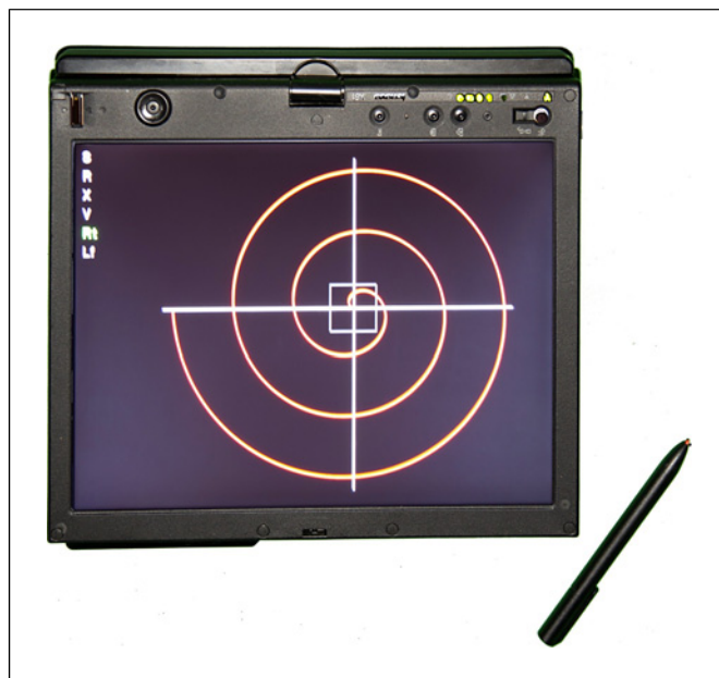
Fig. 1. Photograph of the digital tablet used for collecting spiral drawings.
