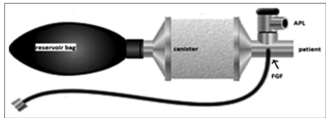
Figure 9: To and fro breathing system
