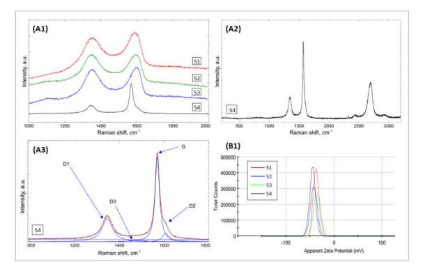
**Figure 3.** Spectroscopic analysis of GO samples. Comparison of the first-order Raman spectra of the S1–S4 samples (**A1**), first and second-order spectrum of the S4 sample (**A2**), and first-order Raman spectra of the S1 sample. The solid line shows the best fit of the sum (red) of four components (G, D1, D2, D3) to the experimental results (black) (**A3**). Electrokinetic potential ( $\zeta$  potential) of the tested GO samples (**B1**).
