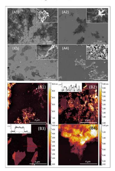
**Figure 1.** Microscopic analysis of tested GO samples. (**A**) SEM analysis: S1 (**A1**), S2 (**A2**), S3 (**A3**), and S4 (**A4**). Scale bars are 10 µm in leading images and 1 µm nm in the inset of the image. (**B**) AFM images: S1 (**B1**), S2 (**B2**), S3 (**B3**), and S4 (**B4**). Scale bars are 4 µm in leading images. An inset on (**B2**) and (**B3**) shows a cross-section through graphene oxide flakes at the marked region.
