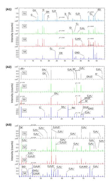
**Figure 4.** Time of Flight-Secondary Ion Mass Spectrometry (TOF-SIMS) of S1–S4 GO samples (**A1–A3**), negative TOF-SIMS spectra narrowed to the 55 Da mass range (**A1**), positive TOF-SIMS spectra in 1–40 Da (**A2**), and 40–80 Da mass range (**A3**).
