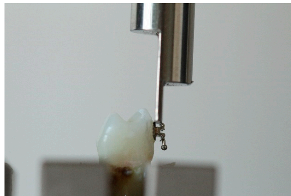
Figure 6. Pin pressing on conventional bracket.
