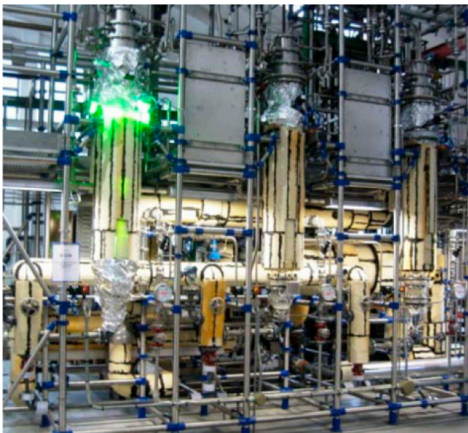
Figure 2. Photooxidation process in semi-synthetic artemisinin ( 1 ) production by Sanofi (Reprinted with permission from [58] Copyright 2016 American Chemical Society).
