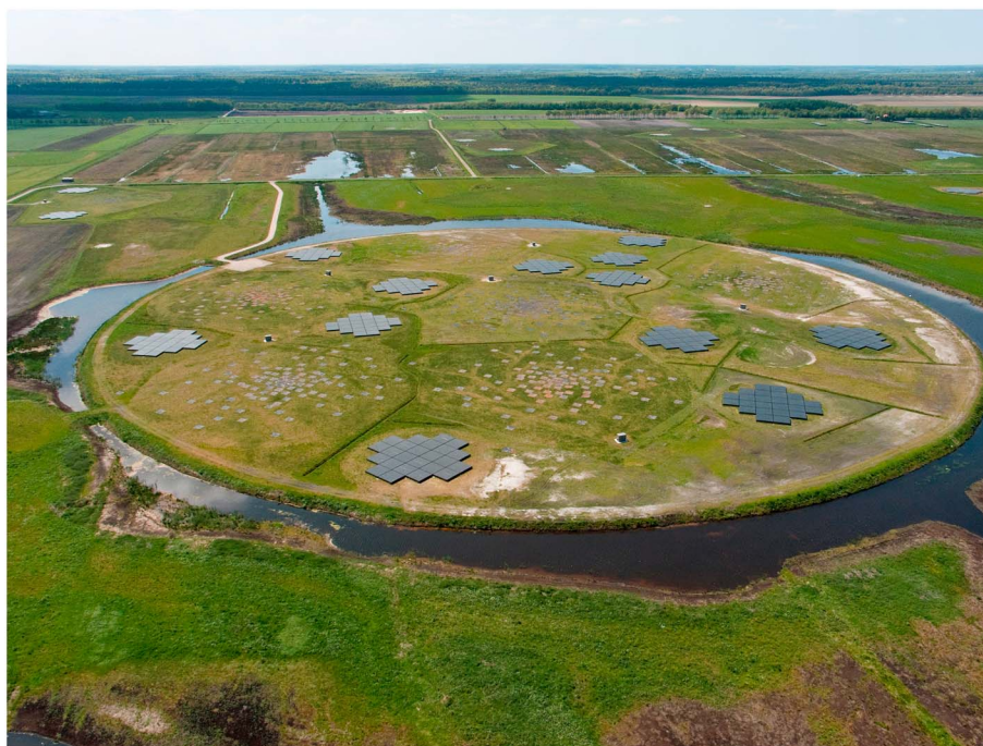
Figure 3. A photograph of the center of LOFAR, called the superterp, which has a diameter of about 370 m. The superterp contains the CS002, CS003, CS004, CS005, CS006, and CS007 stations. The black tiles cover the high-band antennas, and the small gray squares are the low-band antennas. Photo courtesy of ASTRON: https://www.astron.nl/about-astron/press-public/pictures/pictures . ©Top-Foto, Assen
