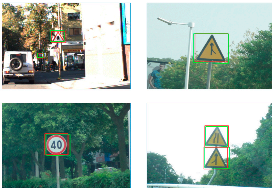
Figure 20. Examples of detection results. The red box represents the traffic signs mark area in the databases, the green box represents the detected areas.
