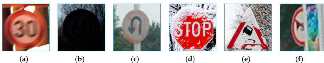
Figure 1. Examples of the unideal traffic sign images: (a) motion blur, (b) undesirable light, (c) color fading, (d) and (e) snow, (f) occlusion.
