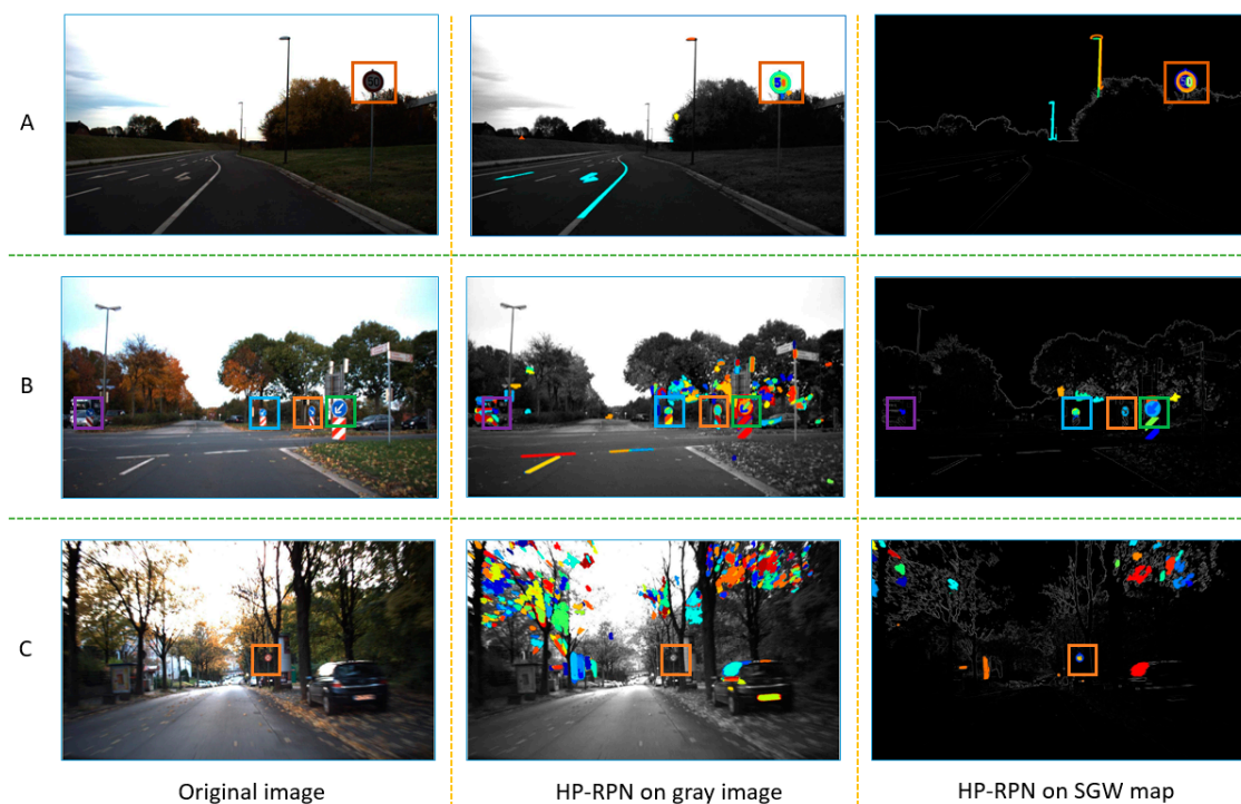
Figure 11. Examples of regions proposal by the highly possible regions proposal network (HP-RPN) on a grayscale image and the HP-RPN on an SGW feature map under different situations of traffic scenes. (A): clear and simple traffic scene, (B): complex traffic scene, (C): motion blurred complex traffic scene.
