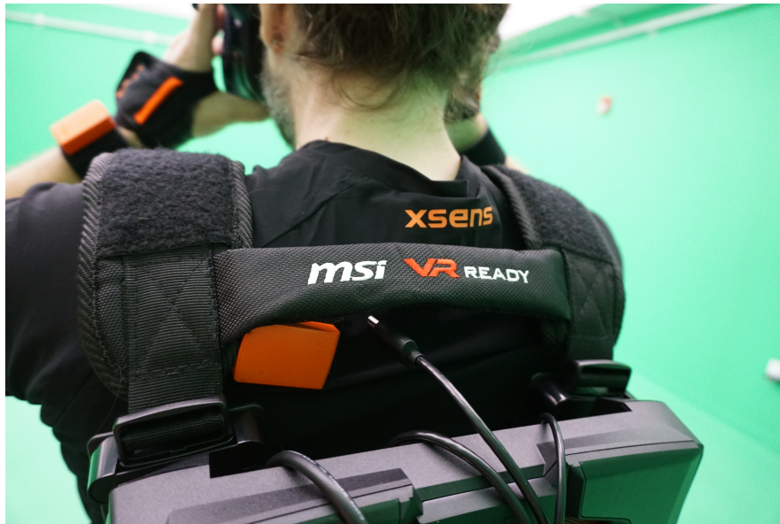
Figure 4. The participant wearing all devices (MSI VR One backpack computer, HTC Vive head-mounted display, and Xsens motion capture system) used for this study.
