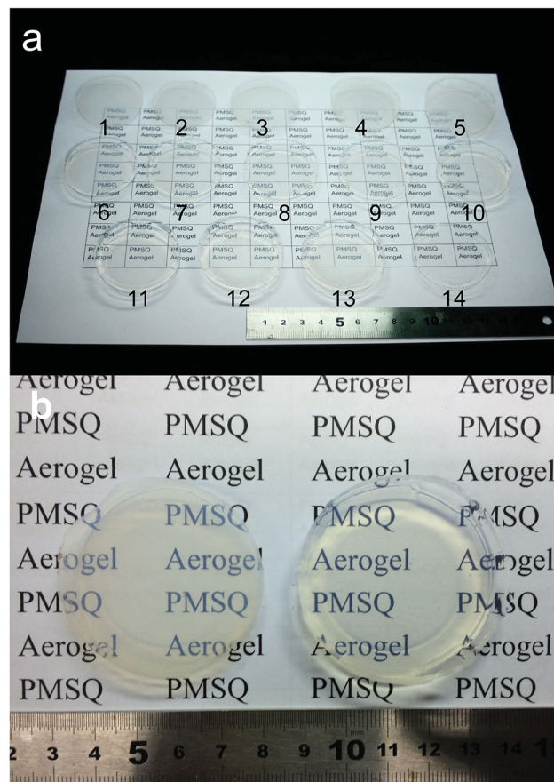
Fig. 1 (a) Fourteen PMSQ aerogels prepared by the proposed method: (1–3) aerogels with densities of \sim 48 mg cm -3 ; (4–5) aerogels with densities of \sim 64 mg cm -3 ; (6–10) aerogels with densities of \sim 84 mg cm -3 ; and (11–14) aerogels with densities of \sim 140 mg cm -3 . (b) Photograph of Modified-7 (left) with a density of \sim 48 mg cm -3 and Modified-4 (right) with a density of 133 mg cm -3 .
