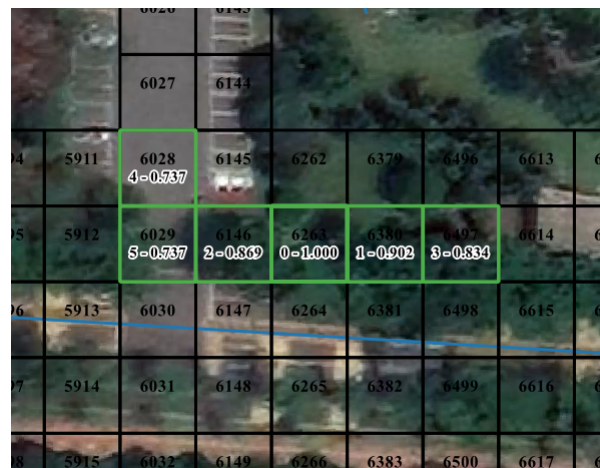
Figure 6. Example of top five proximal cells of CELL6263. “0-1.000” indicates that it is the target cell and the cosine similarity to itself is 1.000. “1-0.902” denotes that CELL6380 ranks 1 in proximal cells, and the cosine similarity to the target cell is 0.902.
