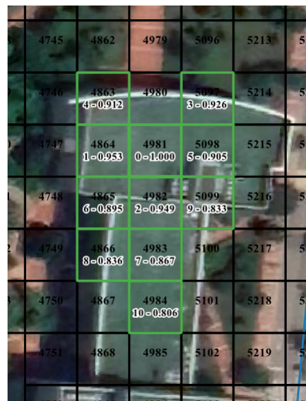
Figure 8. Example of top ten proximal cells of CELL4981. The cells are indoors. “0-1.000” indicates that it is the target cell and the cosine similarity to itself is 1.000. “1-0.953” denotes that CELL4864 ranks 1 in proximal cells and the cosine similarity to the target cell of 0.953.
