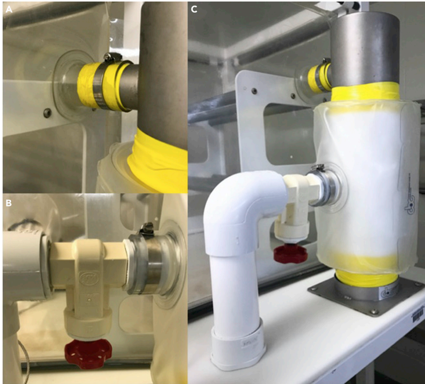
Figure 6. Connecting filters to isolator and air intake/outlet valves
