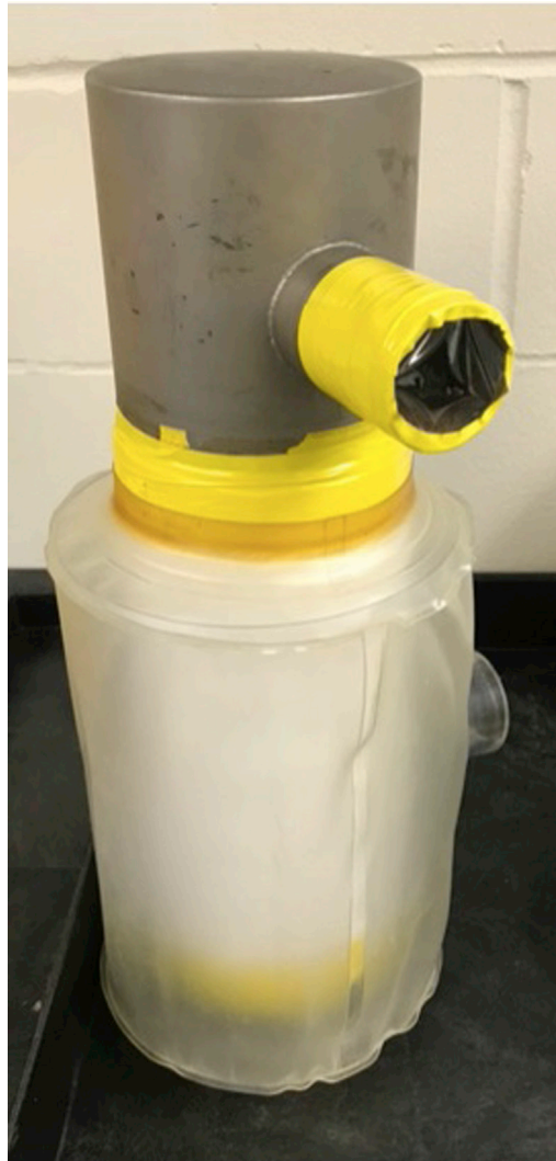
Figure 5. Filter with cover attached with yellow vinyl tape
