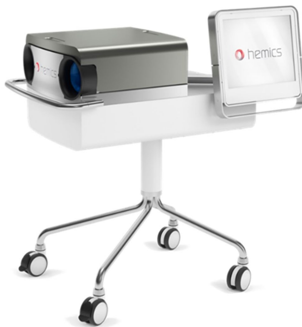
Fig. 1 HandScan. The HandScan (Demcon Hemics, The Netherlands) is a new imaging device for the detection of inflammation. Patients place both hands in the device simultaneously, resting on a plate. Red/near-infrared light illuminates the hand and the amount of light that passes through the hand is recorded by a camera. The more blood is present, the less light is passed through. The total procedure takes approximately 5–10 min and can be executed by any healthcare professional after a short training [15]. The HandScan produces a value for the level of inflammation for each separate joint and a combined score for the entire hand. The inflammation is also shown visually with a scale from green to red superimposed on the joints of the hand and wrists. This may help to understand the current activity of a patient's arthritis as well as to localize inflammatory activity. Previous research showed that the HandScan is a sensitive and specific test with good validity [15, 16]. This makes it interesting to examine the HandScan as a potential addition to or (partial) replacement of current measures for inflammatory activity such as blood tests, DAS28, MRI, and ultrasound
