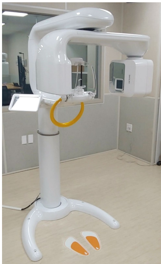
Fig. 1. The newly developed dual-energy cone-beam computed tomography (RCT720, Ray Co., Ltd., Seongnam, Korea) in this study.
