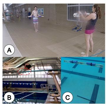
Fig 1. Examining the feasibility of using stereo-video footage collected from the air to measure objects below the water surface. (A) Calibrating the SeaGIS SVC to a custom scale bar before testing. (B) SeaGIS swimmable stereo-video camera on the high dive, stereo-video camera in red dashed outline. (C) Underwater scale bar testing mechanism at 5.0 m depth. Testing was conducted at the University of West Florida Aquatic Center.
