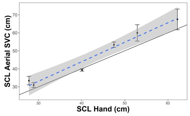
Fig 7. Comparison of hand measurements to SVC-UAV for green sea turtles (n = 6) from the field trial in Eleuthera, Bahamas. The dashed line and gray shaded area are the linear regression and standard error, respectively. The solid black line is the 1:1 line for the hand and SV-UAV measurements; points that fall on this line have equivalent measurements for both methods.
