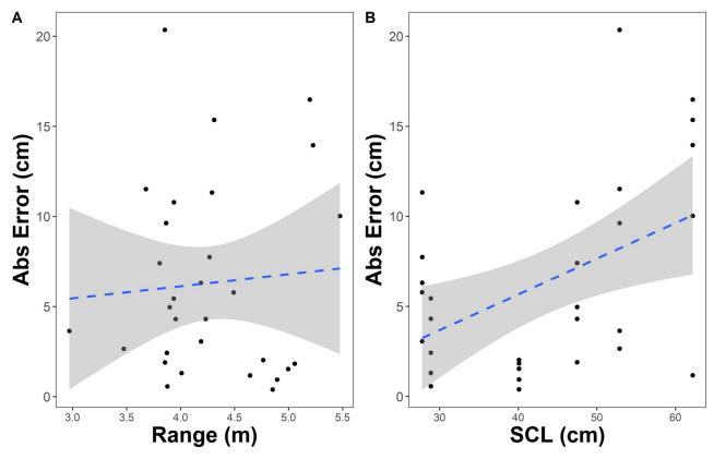
Fig 8. Relationship between absolute error and (A) range and (B) straight carapace length from the stereo-video camera system mounted to an **unoccupied aerial vehicle**. The dashed line and gray shaded area are the linear regression and standard error, respectively.
