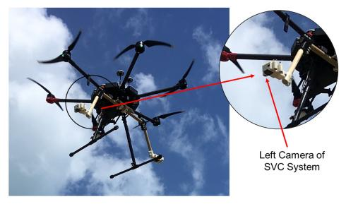
Fig 3. Unoccupied aerial vehicle in flight with stereo-video camera system mounted, and left camera highlighted. https://doi.org/10.1371/journal.pone.0276382.g003
