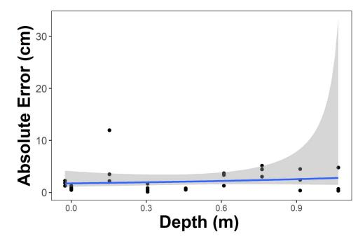
**Fig 6. Relationship of absolute error of aerial SVC measurements and depth.** The solid line and gray shaded area are the generalized linear regression and standard error, respectively. Depth measurements of <0 indicate measurements made from the camera in the air only, just above the water surface.
