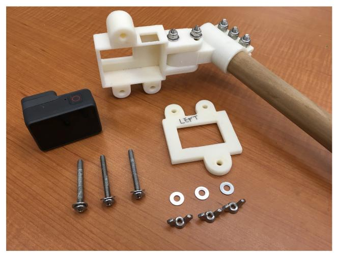
Fig 4. Stereo-video camera housing. Custom ABS plastic 3D printed housing, which allows access to camera functions for the GoPro Hero 5 Black camera. Housing is fastened using stainless steel screws and wingnuts for corrosion resistance.
