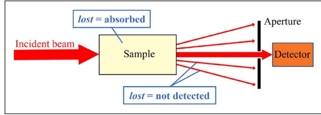
**Figure 5.** Example of a simple setup used to measure the unscattered light intensity, also called coherent or ballistic component, that arise from the propagation of a collimated light beam through an absorbing and weakly scattering media. The usage of an aperture allows for the detection of only the unscattered light.
