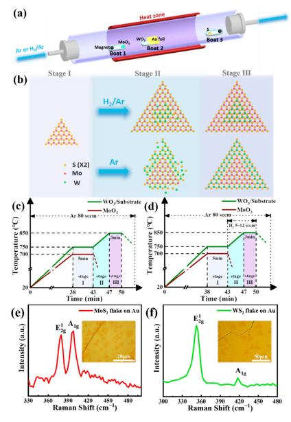
Figure 1. (a) Schematics of the CVD setup for the growth of  $WS_2/MoS_2$  LHs and VHs; (b) schematic illustrations of  $WS_2/MoS_2$  LHs and VHs growth process; (c,d) temperature program of the CVD growth process for  $WS_2/MoS_2$  LHs and VHs, respectively; (e,f) Raman spectra of as-grown  $MoS_2$  and  $WS_2$  monolayers, respectively. Insets: Corresponding optical microscopic images of the  $MoS_2$  and  $WS_2$  flakes on Au foil.
