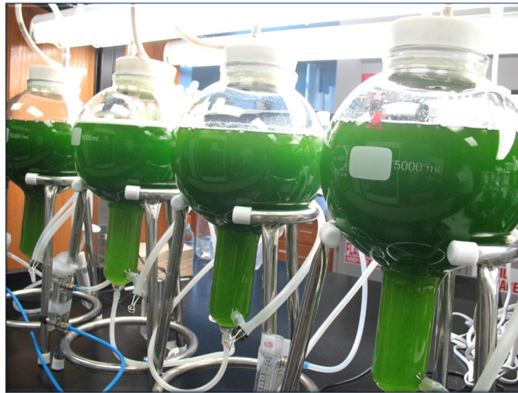
Figure 4 Biomass production of S. bacillaris strain siva2011 in 5 L balloon type bioreactors (working volume 4 L).
