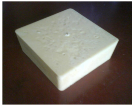
Figure 1. A rigid PU foams' block, molded in a sealed steel mould.
