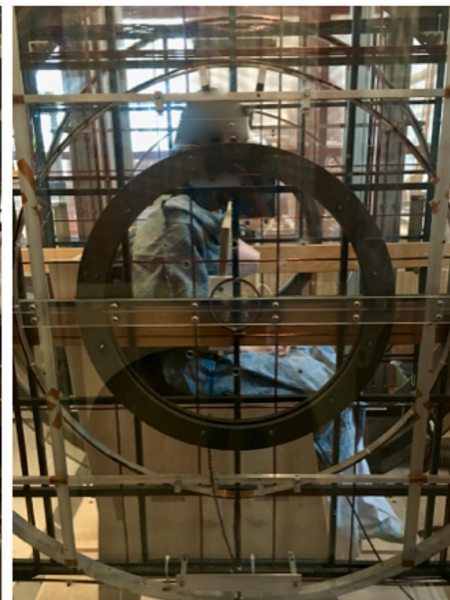
Fig. 1. Experimental setup for single left breast imaging using an ultra-low field (ULF) MRI scanner at 6.5 mT. (a) ULF MRI B_0 coils of the resistive electromagnet are shown on each side of the table with an open design. A wooden table was positioned at the center of the scanner for imaging in the prone position. The gray arrow indicates the transmit/receive radiofrequency (RF) coil, which is embedded in the table. (b) A wooden chair was designed to fit inside the magnet for imaging in the seated position. A single breast RF coil is attached to the wooden frame (gray arrow). A volunteer is shown from the side view in the prone (c) and seated (d) positions.
