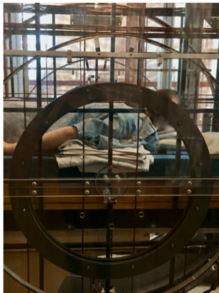
Fig. 1. Experimental setup for single left breast imaging using an ultra-low field (ULF) MRI scanner at 6.5 mT. (a) ULF MRI B_0 coils of the resistive electromagnet are shown on each side of the table with an open design. A wooden table was positioned at the center of the scanner for imaging in the prone position. The gray arrow indicates the transmit/receive radiofrequency (RF) coil, which is embedded in the table. (b) A wooden chair was designed to fit inside the magnet for imaging in the seated position. A single breast RF coil is attached to the wooden frame (gray arrow). A volunteer is shown from the side view in the prone (c) and seated (d) positions.
