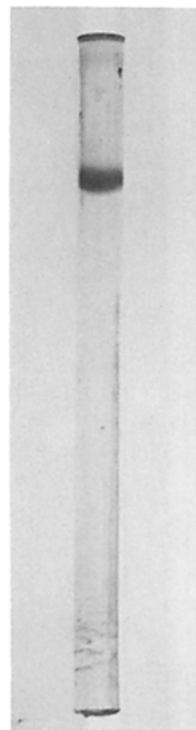
FIGURE 1 SDS-polyacrylamide gel electrophoresis of purified chicken AMP deaminase prepared by the method of Smiley et al. (22). The gel was loaded with 100 \mu g of enzyme and stained with Coomassie brilliant blue.
