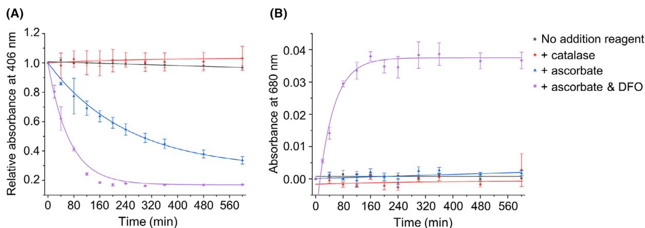
**Fig. 2.** Characterization of coupled oxidation. The absorbance difference at 406 nm of heme-AtHO-1 (A) and at 680 nm of biliverdin (B). Additions of catalase, ascorbate, and ascorbate with DFO are shown in red, blue, and purple, respectively. Error bars represent the standard deviation from three independent measurements.
