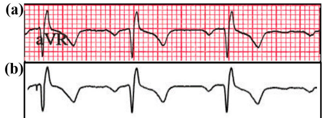
FIGURE 9. Digitization of scanned paper ECG samples with the inclusion of character removal. (a) The original ECG waveform is displayed containing the ECG lead character "aVR". (b) ECG waveform is digitized, with the ECG lead character 'aVR' removed during the process of digitization.
