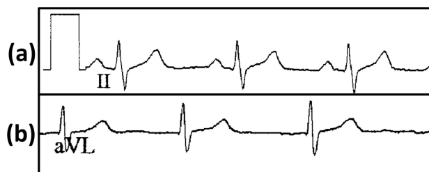
FIGURE 6. The ECG records after thresholding and grid removal are displayed to illustrate the issue of overlapping text on ECG signals. (a) The ECG lead character 'II' is well separated from the ECG signal. (b) The ECG lead character 'aVL' overlaps the ECG signal.
