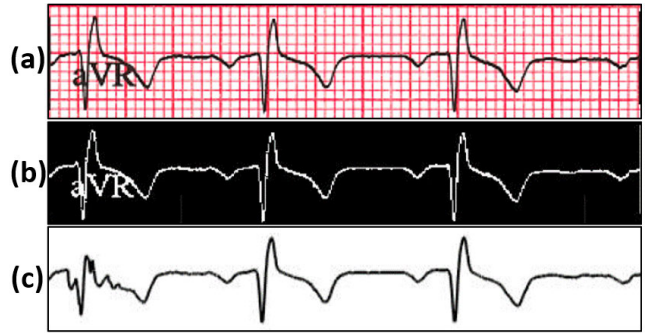
FIGURE 8. The intermediate results are shown sequentially for the ECG digitization process. (a) Sample paper ECG record without any processing; (b) Image obtained after application of thresholding and filtering; (c) Digitization of ECG segment without ECG lead character removal using column pixel scanning.
