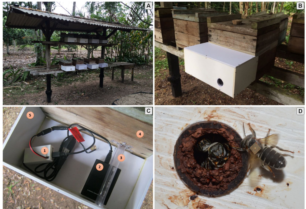
Figure 1. The system environment. (a) The eight M. fasciculata hives employed in this study. (b) Frontal view of the adapted hive entrance: it contains a PVC box for storing electronic items. (c) Electronic system details: (1) Intel Edison TM for RFID reader control and data storage, (2) USB RFID reader, (3) Transparent hose where the bees pass upon the RFID reader, (4) Hive of M. fasciculata , and (5) PVC box. (d) Tagged M. fasciculata at the hive entrance.
