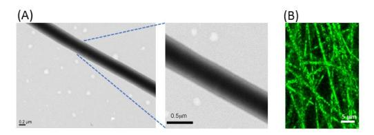
**Figure 3.** The transmission electron microscope (TEM) (**A**) and the confocal laser scanning microscope (the core solution was labeled with fluorescein isothiocyanate) (**B**) micrographs of polylactic acid/docosahexaenoic acid (PLA/DHA) core-shell nanofibers.
