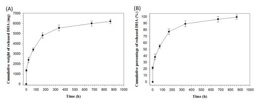
**Figure 5.** The release profiles of docosahexaenoic acid (DHA) from polylactic acid/docosahexaenoic acid (PLA/DHA) core-shell nanofiber membrane determined from the cumulative released weight (**A**) and cumulative released percentage (normalized to loaded DHA in the membrane) (**B**) of DHA.
