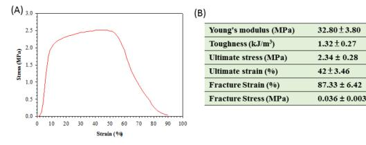
**Figure 4.** A typical tensile stress–strain curve of polylactic acid/docosahexaenoic acid (PLA/DHA) core-shell nanofiber membrane (**A**) and parameters of mechanical property determined from the stress-strain curves (n = 6, mean  $\pm$  SD) (**B**).
