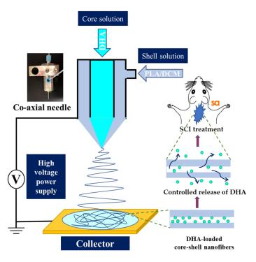
**Figure 1.** The schematic diagram showing the preparation of docosahexaenoic acid (DHA)-loaded core-shell nanofibers using polylactic acid/dichloromethane (PLA/DCM) shell solution for the treatment of spinal cord injury (SCI) in rats.
