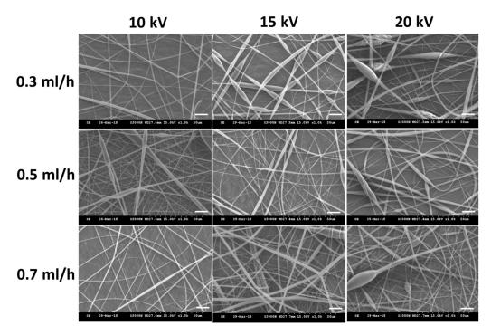
**Figure 2.** The scanning electron microscope (SEM) images of the electrospun polylactic acid/docosahexaenoic acid (PLA/DHA) core-shell nanofibers fabricated under different voltage (in kV) and core solution flow rate (in mL/h).
