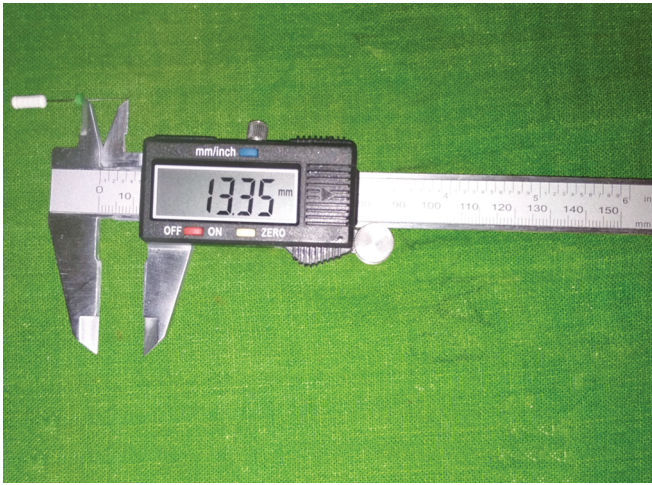
Fig. 2: File length measurement using a digital Vernier caliper
