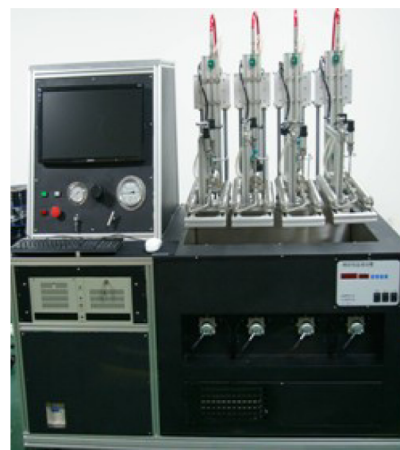
Figure 2. Schematic of the methane adsorption and desorption measurement apparatus for coal.
