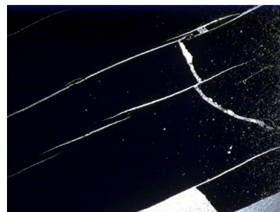
Figure 10. Cleats and fractures of a coal cast thin section under 25\times magnification. 15 Reprinted with permission from [Huang, W. A.; Lei, M.; Qiu, Z. S.; Leong, Y. K.; Zhong, H. Y.; Zhang, S. F. Damage mechanism and protection measures of a coalbed methane reservoir in the Zhengzhuang block. J. Nat. Gas. Sci. Eng. 2015, 26, 683–694]. Copyright [2015] [Elsevier].
