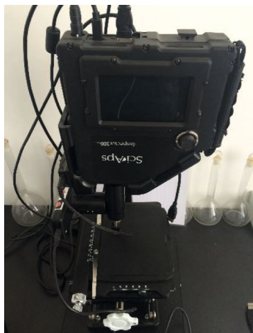
FIGURE 1: Portable Raman system for on-line measurements of meat consisting of a hand-held Raman device.
