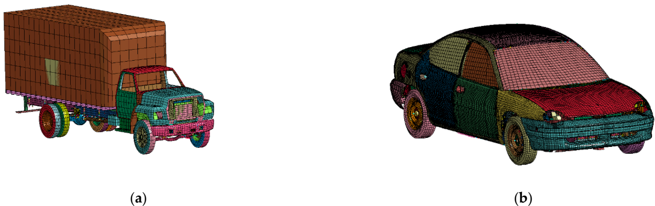
Figure 7. Three-dimensional view of the FE model: (a) a Ford single unit truck and (b) a Dodge Neon.
