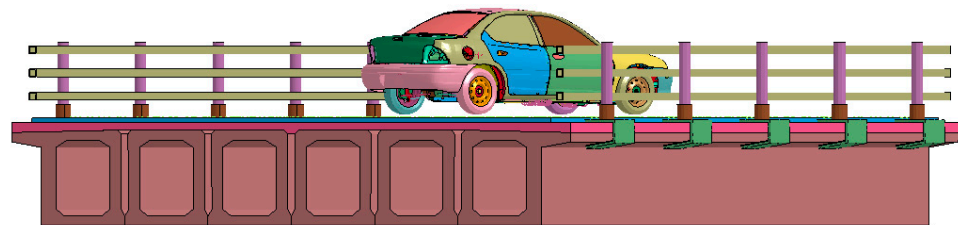
Figure 4. Car and bridge finite element 3D model.
