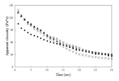
**Fig. 1. A Change in apparent viscosity of meat batter containing different levels of lotus rhizome powder for 30 s.** (♦) meat batter without lotus rhizome powder; (□) meat batter with 1% lotus rhizome powder; (▲) meat batter with 2% lotus rhizome powder; (×) meat batter with 3% lotus rhizome powder.
