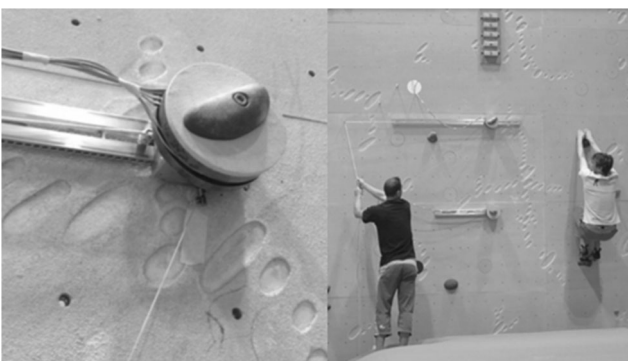
Fig. 2 ledge mechanism to slide the targeted hold (left) and start position for distance estimation (right)
