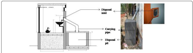
Fig. 2 Piloted and implemented chute disposal system in pilot and implementation schools of Dhaka and Manikganj (Source: DSK and icddr,b, permission obtained from DSK to use the chute disposal design)
