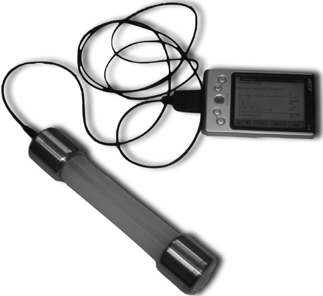
Figure 1. The Painmouse®. The measuring device connected to a hand-held portable computer. doi:10.1371/journal.pone.0051014.g001
