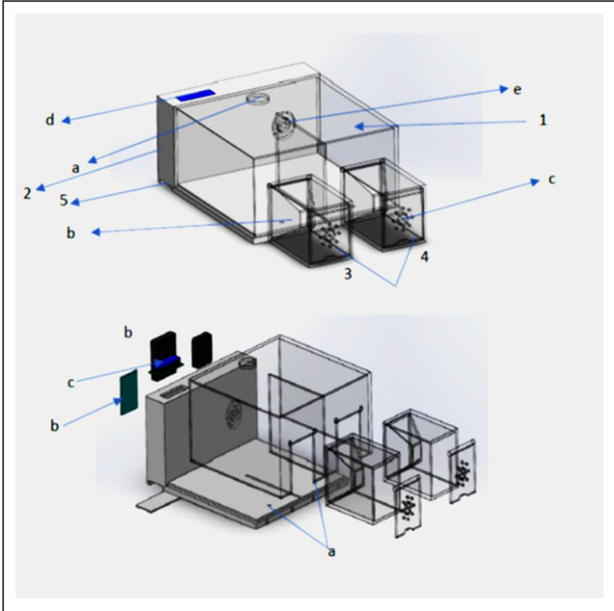
**Figure 1.** A, olfactometer 2.0 front view, 1: Box; 2: base; 3: control chamber; 4: test chamber; 5: sliding door; a: central hole; b: funnel; c: holes; d: LCD monitor, an arduino, e: Fan. b, exploded view, a: Sensors, b: Arduino, c: LCD screen.
