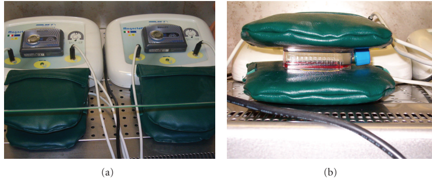
FIGURE 2: The apparatus used to generate the ELF EMFs and TAMMEFs (a). Cells were exposed to EMFs for 30 minutes (b) at room temperature.
