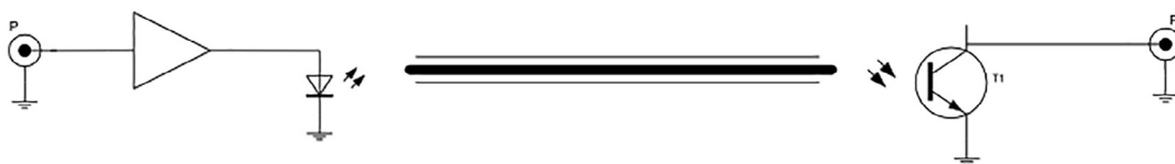
Fig. 4. Optical communication scheme. A TTL signal comes out of a digital Arduino port, is amplified, and converted into light through a LED. The light is transmitted through an optical fiber to the terminal where it will be converted into a TTL signal.
