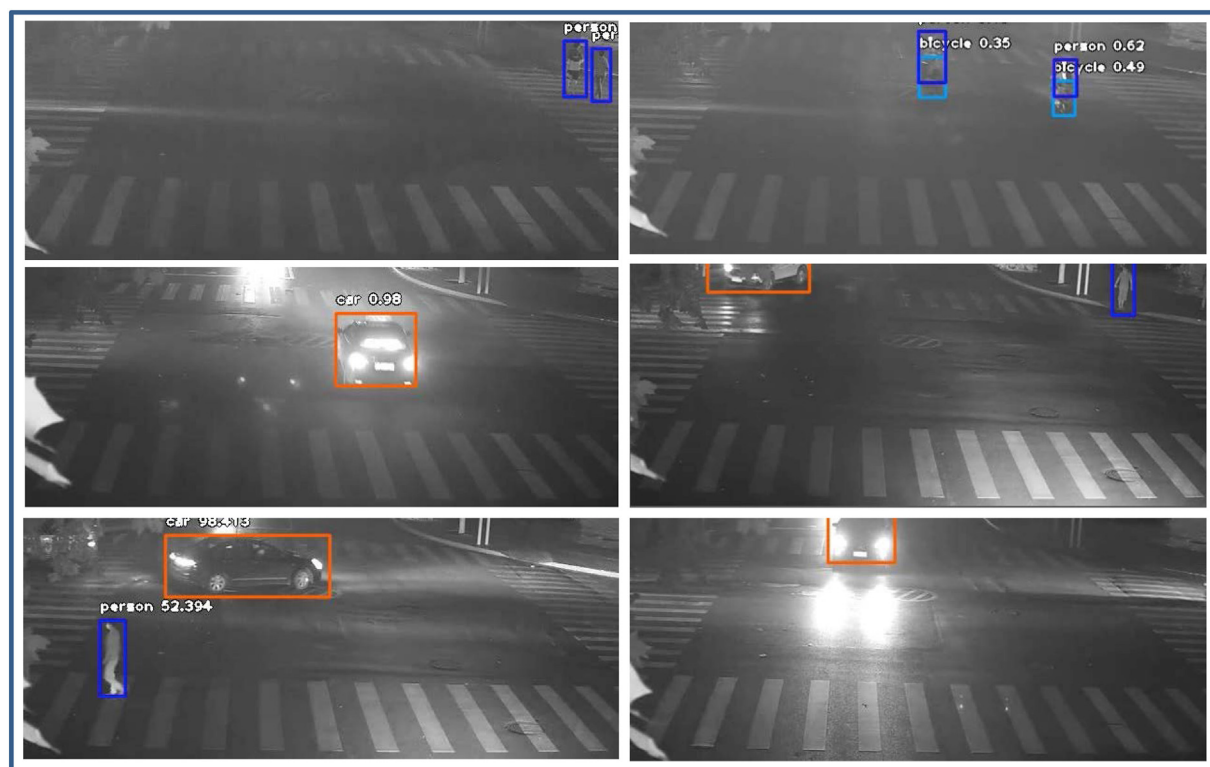
Figure 6. Detection results by the presented framework in the presence of significant interference.
