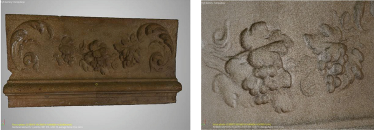
Fig. 5. Reconstruction of the object after cleaning and the density of the point cloud
