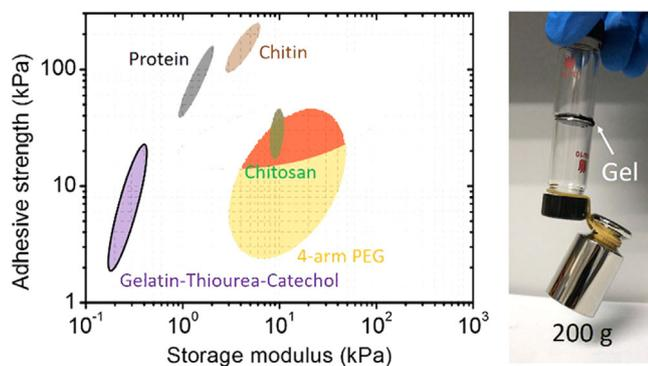
**FIGURE 24** Adhesive strength versus storage modulus for different biomaterials<sup>284</sup>
