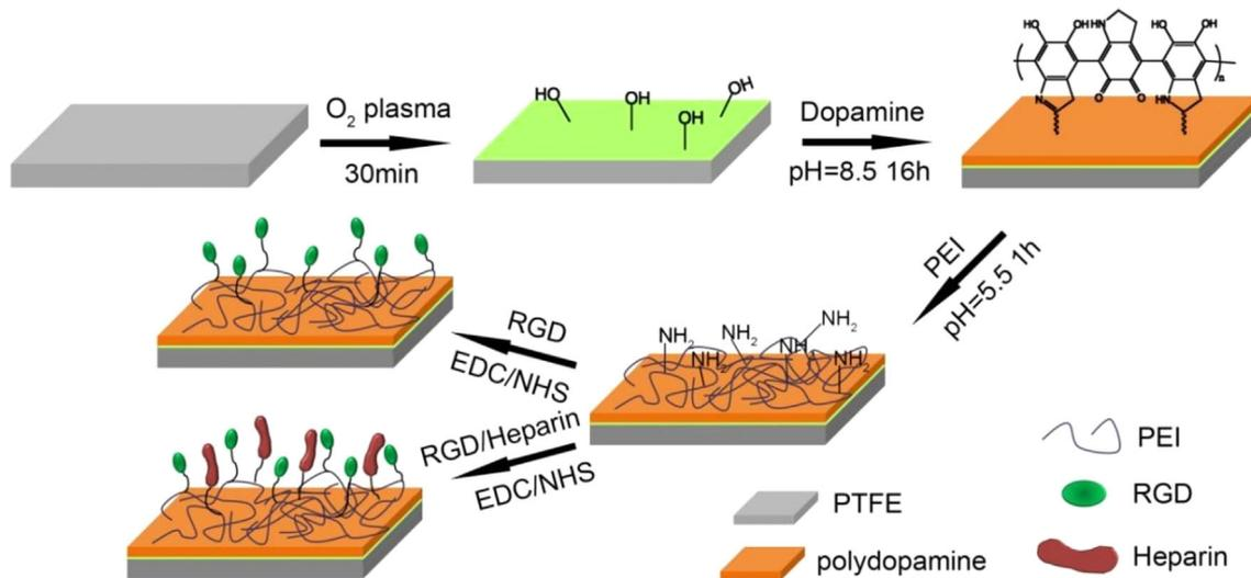
**FIGURE 25** Schematic immobilization of RGD/heparin on dopamine/polytetrafluoroethylene film<sup>309</sup>
