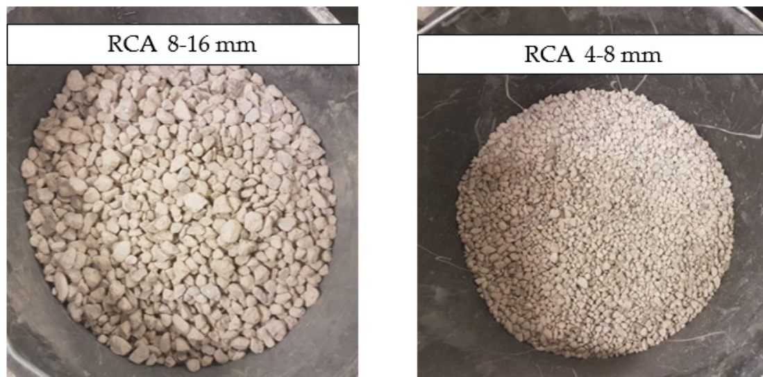
Figure 1. Recycled concrete aggregate (RCA): 8–16 mm fraction (on the left) and 4–16 mm fraction (on the right).
