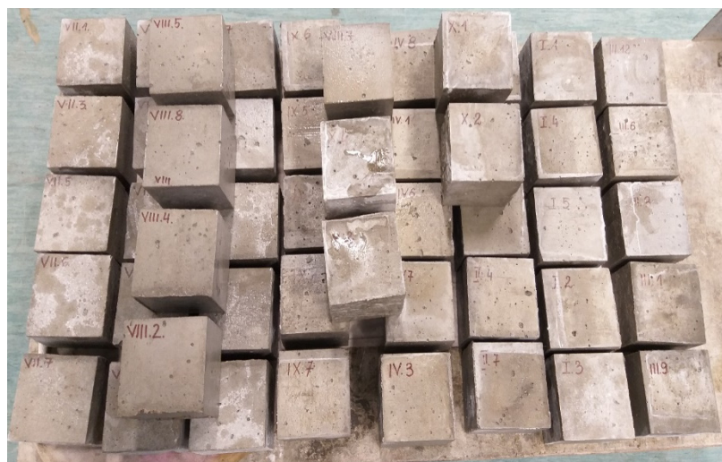
Figure 4. Concrete cubes prepared for testing.
