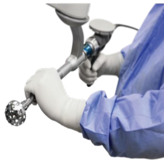
Figure 9. MAKO robotic arm attached to an acetabular reamer to provide feedback and guide surgical reaming of the acetabulum intraoperatively.
