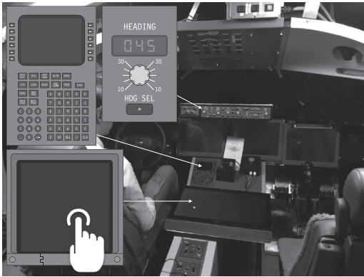
Figure 3. Cabin of the SIMONA Research Simulator (SRS) showing each of the three flight deck interfaces.
