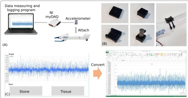
Fig. 1 Depiction of the data collection system. a Illustration of the overall acceleration measure system. b Accelerometer and its mount attached to an endoscope. c Data storage and conversion with the data measuring program
