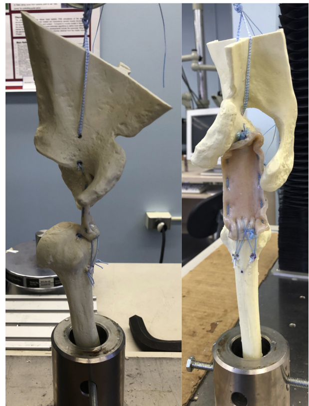
Fig 3. Biomechanical testing setup shown using a reinforced HD allograft; left shows side-view of testing setup; right shows front-view of testing setup. (HD, human dermal.)
