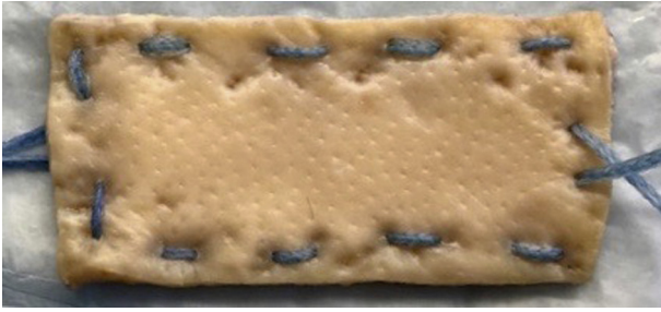
Fig 2. Suture-reinforced HD allograft before testing. The graft is shown before tying of sutures at medial and lateral edges to better illustrate the use of the 2 sutures used. (HD, human dermal.)
