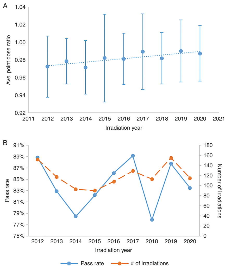
Figure 2. a) The average measured to delivered point dose (average TLD ratio) value for the SRS phantom through the years b) Pass rates for the SRS head phantom through the years with an overall average of 84.6% (solid line) combined with the number of irradiations performed per year (dashed line). The error bars presented in graph a represent \pm one standard deviation. There has been an overall increase in point dose performance relative to a site's dose calculation but passing rates have remained constant over the span of our data set.
