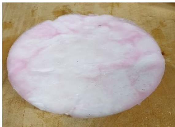
Figure 8. Hydrate pellet obtained from pressing after hydrate formation (at 37.5 bar and 3 °C) in the water–sucrose–betanin model solution.
