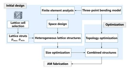
Figure 2. The design flow of heterogeneous lattice structures in this work.
