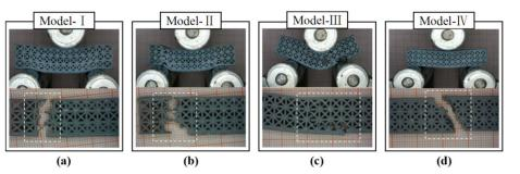
**Figure 11.** The failure modes of the proposed lattice structures: (**a**) Heterogeneous lattice No. 1, (**b**) Heterogeneous lattice No. 2, (**c**) Uniform model with FCC strut diameter of 0.8 mm, (**d**) Uniform model with FCC strut diameter of 1 mm.
