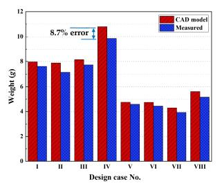
Figure 8. The weight of the eight types of lattice samples compared to their CAD models.
