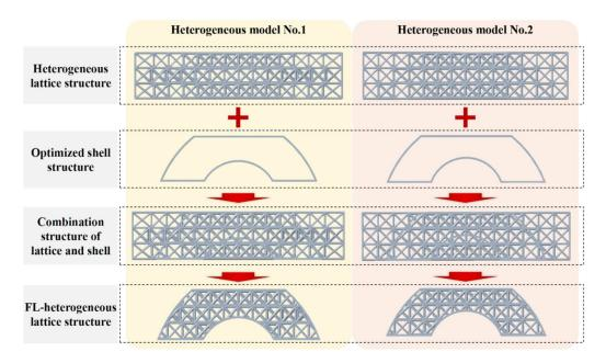
**Figure 6.** The schematic of the generation process of topology-optimized lattice structures for further weight reduction under the load-bearing orientation and stress distribution.
