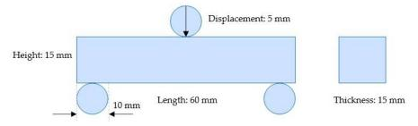
Figure 1. Geometric boundary conditions of the verification part for FEA.
