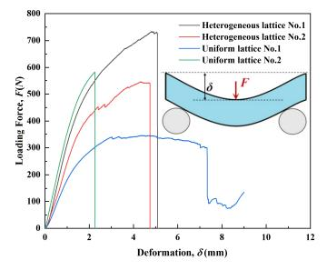
Figure 9. The bending load-displacement curves of the four lattice structures.
