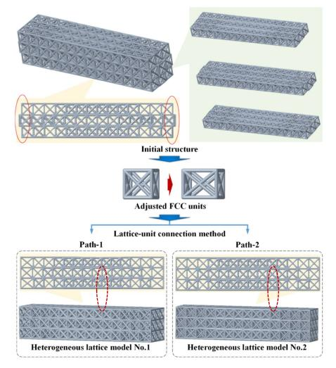
Figure 4. The design flow of the two structural optimization paths.
