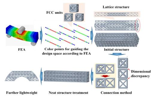
Figure 3. The initial design of the hybrid structure.
