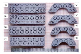
**Figure 7.** Eight types of lattice samples via SLA for three-point bending: (**I**) Heterogeneous lattice No. 1, (**II**) Heterogeneous lattice No. 2, (**III**) Uniform lattice No. 1, (**IV**) Uniform lattice No. 2, (**V**) FL-heterogeneous lattice No. 1, (**VI**) FL-heterogeneous lattice No. 2, (**VII**) FL-uniform lattice No. 1, (**VIII**) FL-uniform lattice No. 2.
