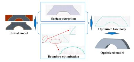
**Figure 5.** The schematic of the generation process of the topology-optimized model for further solid-body weight reduction under the load-bearing orientation and stress distribution.
