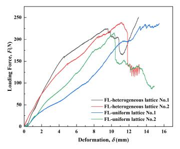
Figure 10. The bending load-displacement curves of the four lattice hybrid structures.
