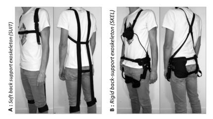
are attached to shoulder straps at the upper ends, and under the knees at the lower ends (Figure 2A).
