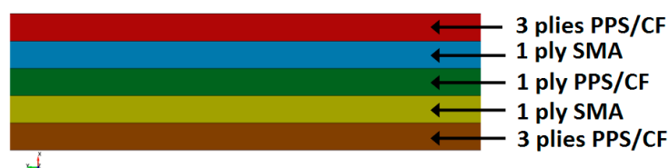
Figure 9. Layup configuration of the simplified model.
