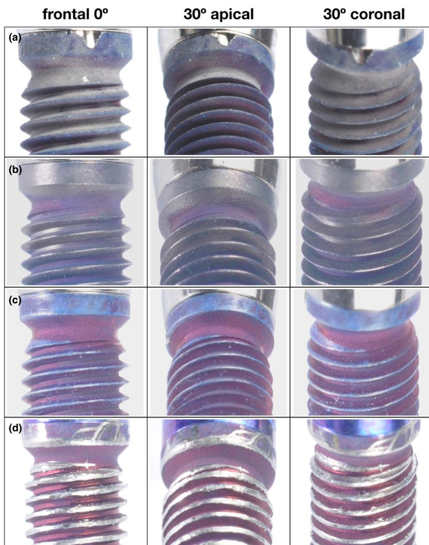
FIGURE 3 Picture samples from different points of view of the implants treated with different devices. AF group (a), TB group (b), PI group (c), US group (d).
